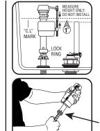
Position fill valve in tank, but do not fully install vet. Top of fill valve MUST be set 3" above overflow pipe. This will automatically place CRITICAL LEVEL MARK / C.L. Mark, 1" above the top of overflow pipe. Remove fill valve from tank to adjust height.
