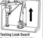
Simulate a leak by slightly lifting flapper chain to allow 3 or 4 inches o water to slowly drain from tank. Fill valve should not turn on, but remai locked and stav off
