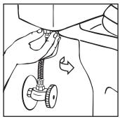
12. Reconnect water supply line to bottom of toilet fill valve
