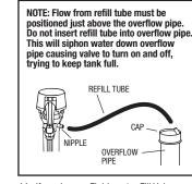
11. If you have a Fluidmaster Fill Valve, remove overflow pipe ring. Then use cap to attach directly to refill tube.
