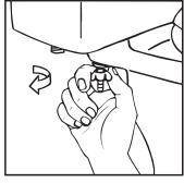
2. Unbolt tank from bowl, then lift off tank. Remove washers and nuts from bottom of tank, then remove old bolts. Remove old
