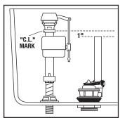
4. When installed, the top of the overflow pipe on the new flush valve should be at least 1" below the hole in the tank where the tank flush lever is mounted. If necessary, cut the overflow pipe with saw to achieve this height. The critical level mark on the fill valve (identified by a C.L. mark on the Fluidmaster Fill Valve) should be at least 1" above the top of the overflow pipe.
