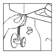
1.Turn off water supply. Flush toilet and remove excess water from tank with sponge. Remove water supply line from bottom of toilet fill valve.
