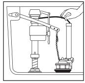
Attach existing refill tube to overflow nine.
