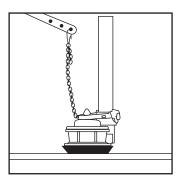
**9.**Connect flapper chain. Allow slight slack when flapper is in closed position.
