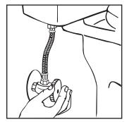
13. Turn on water supply, check for leaks,
