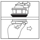
5. Install new flush valve. Tighten lock nut 1/2 turn beyound hand tight. DO NOT OVERTIGHTEN or tank may crack.
