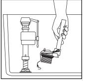
**3**. Remove old flush valve, including flapper/tank ball unit.
