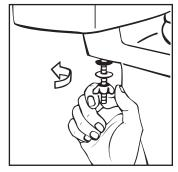
8. Reconnect tank to bowl with bolts, washers and nuts. Tighten bolts evenly, DO NOT OVERTIGHTEN or bowl may crack.
