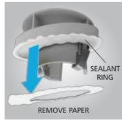
**Step 5**: Remove the paper from SEALANT RING located on the bottom of the ANGLED SEAT ADAPTER. DO **NOT REMOVE SEALANT** RING from the adapter.
