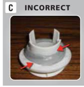
**C**: Sealant ring pressed too hard and high against the adapter wall causing it to deform from its original shape – this will not provide adequate coverage on the surface of the adapter as shown with arrows.
