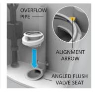
Step 6: Locate yellow arrow on back of the ANGLED SEAT ADAPTER. Align yellow arrow on ANGLED SEAT ADAPTER directly toward the plastic OVERFLOW PIPE and push the ANGLED SEAT ADAPTER onto the FLUSH VALVE SEAT. As the adapter is firmly pressed onto the FLUSH VALVE SEAT, the SEALANT RING located on the bottom of the ANGLED SEAT ADAPTER will spread to provide correct coverage and seal.
