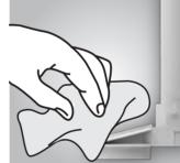
Step 4: Prior to installing the ANGLED SEAT ADAPTER, use warm soapy water and scrub pad to clean the existing FLUSH VALVE SEAT. Then dry the seat and the area around it on the bottom of the tank.
