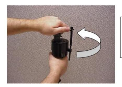
The bottom hand is lifting up on the float cup which raises the black arm under the top cap. The top hand is gripping the cap while the thumb is pressing on the raised lever arm.
