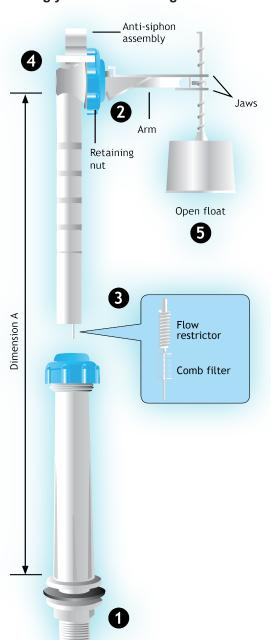
Fit the Torbeck filling valve ensuring the rubber washer is on the inside of the tank with the conical side face down. Hand tighten the back nut and with a spanner, tighten a further three-quarter turn.
