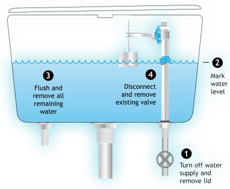
Valve can be fitted on either side of the cistern
