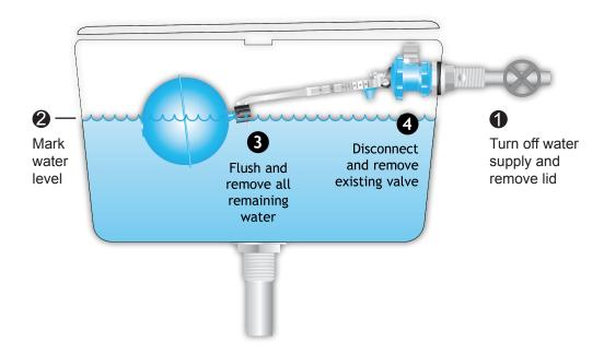
Valve can be fitted on either side of the cistern
