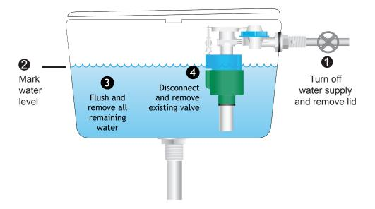
Valve can be fitted on either side of cistern.
