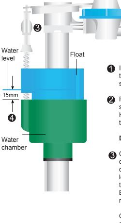
Insert correct filter restrictor into threaded tail (see overleaf for correct flow restrictor settings).
