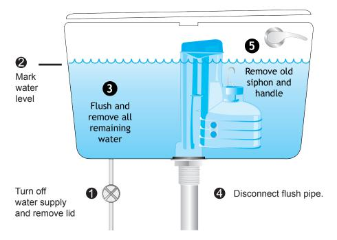
**Note:** Ensure the top of the new variflush valve is below the lowest overflow point of the cistern including all apertures.
