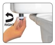
F: ATTACH REFILL TUBE TO REFILL CLIP Note: If refill tube is too long, cut tube.
