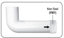
C: Fit Flush pipe coupling nut and double cone washer wedge seal onto flush pipe. Hand-tighten Flush pipe coupling nut and secure flush pipe to outlet valve shank. DO NOT OVERTIGIHEN
