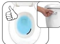
If the water level matches the line in the bowl and the fill valve is **STILL FILLING**, then the bowl water is **TOO HIGH**, proceed to Step 7D.
