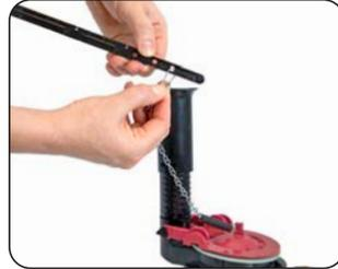
To adjust chain length, remove clip and reposition lower on the chain for shorter length.
